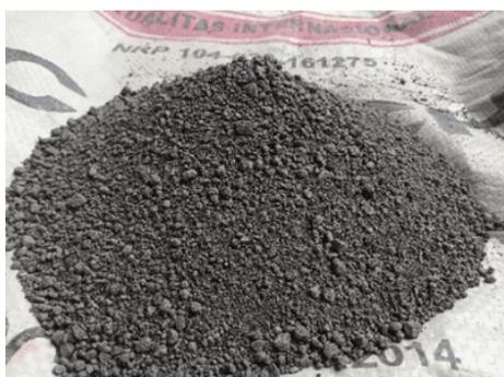
**Gambar 3.** Agregat Halus Pasir Kalumata
